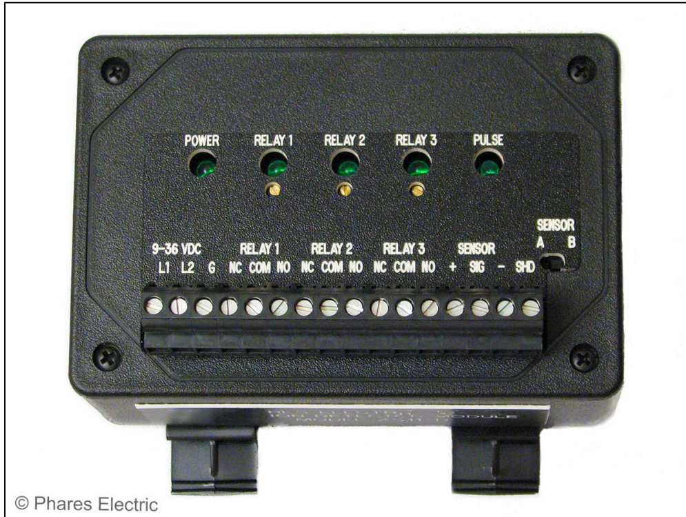
Figure 1. Indicators and Terminal Block
