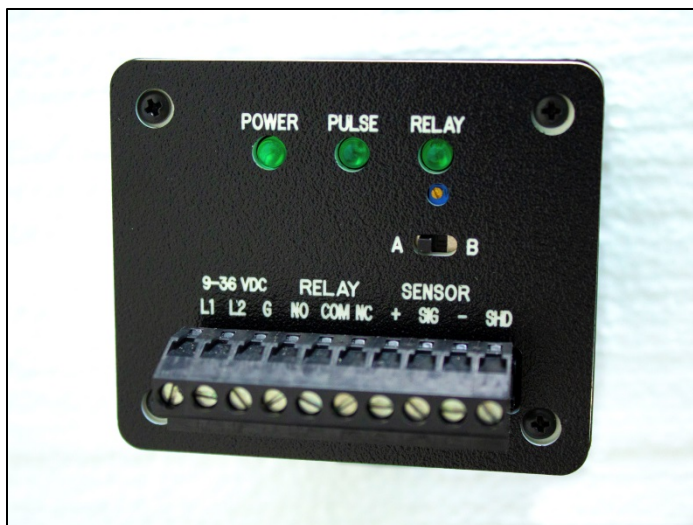
Figure 1. Indicators and Terminal Block.
