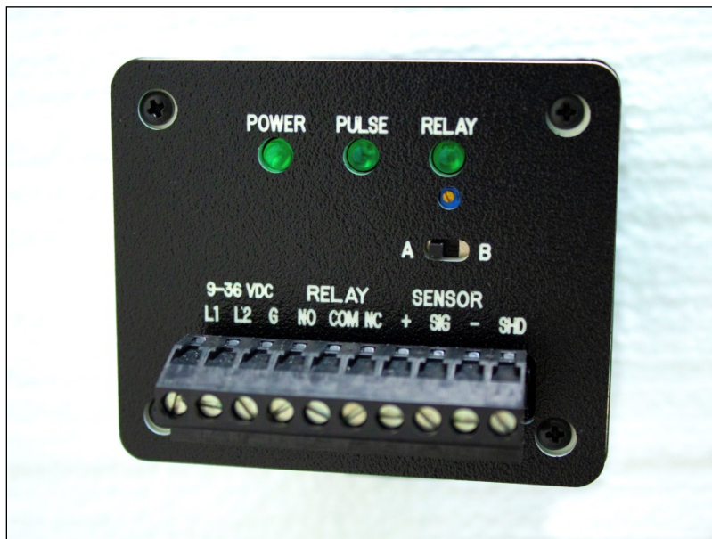
Figure 2. Indicators and Terminal Block (ZS10-D Shown)
